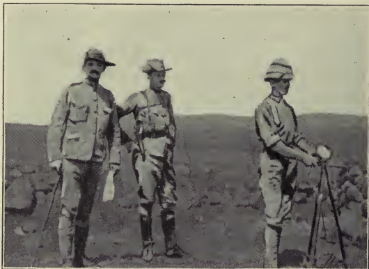
Major Nylén, Cape Mounted Police, and Captain Tennant, Third Divisional Intelligence Officer and Press Censor, Heliographing from Cyphergat to Sterkstroom. The mirror reflecting the sun's rays can flash signals eighty miles. The Morse telegraphic code is used.
